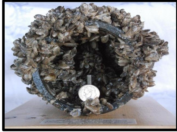
Colonized pipe after 3 months exposure
